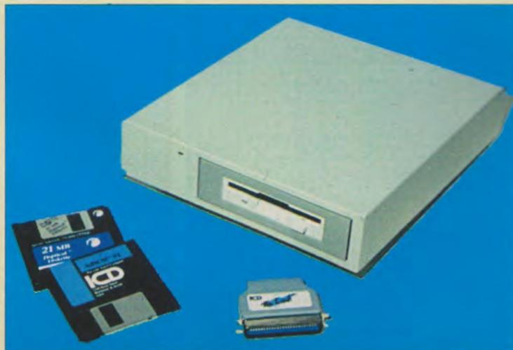
*The Link enables ST owners to use industry standard SCSI drives and other devices such as the Floptical drive shown here. It simply plugs into the back of the ST; a single Link can be used to chain up to eight devices.*
