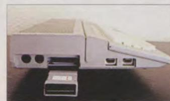
*The ST's cartridge port is often used for connecting a clock or a copy protection "dongle".*
