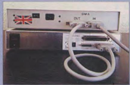
*Daisy-chaining two hard disk drives. The top is drive 0 and the bottom drive is designated as drive 1.*
