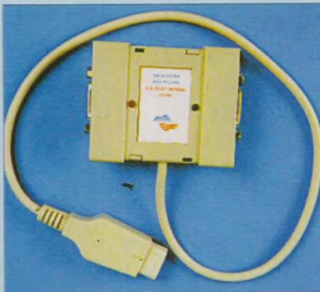
**A mouse/joystick port switcher is convenient and prevents costly port damage.**
