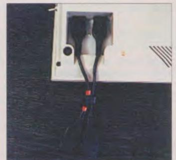
*The mouse/joystick ports are not in the best place on the ST but an extension lead can help.*
