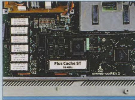
**Plus Cache 16 is an easier upgrade path than trying to replace the 68000 with a 68010.**
