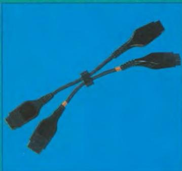
Either a single or twin joystick adaptor will save you from the ST's most common hardware fault - a broken mouse port. Changing from mouse to joystick is that much easier if you have extension cables.
